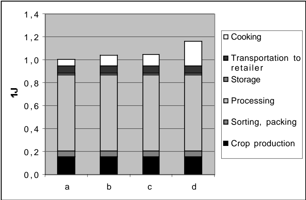
Figure 10: Energy use during the life cycle of one portion of mashed potatoes from mashed potato powder. In MJ per portion according to cooking mode. Example a was cooked with an electric kettle as part of 4 portions, example b as a single portion with an electric kettle, example c on a hotplate as part of 4 portions and example d on a hotplate as a single portion.
